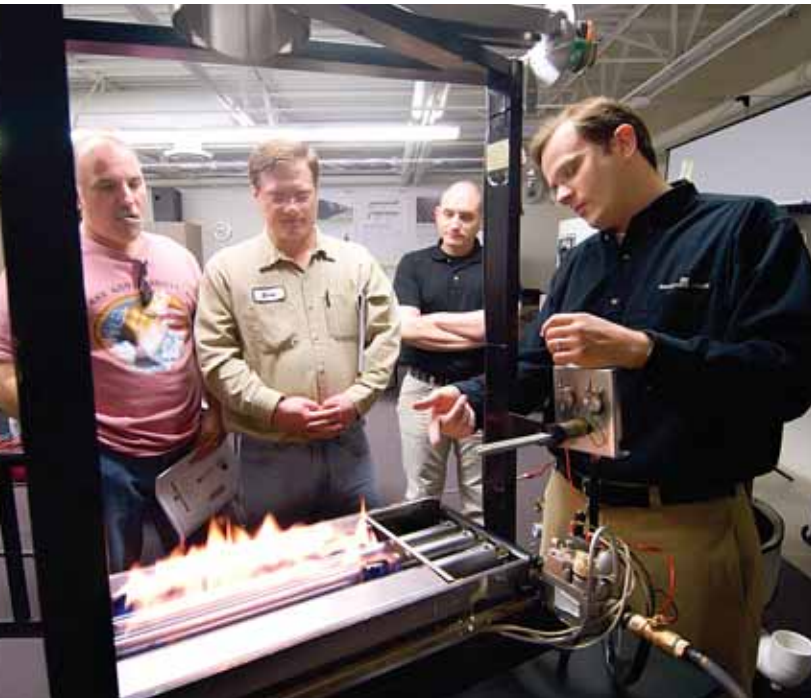
Rick Michel, with an operating cutaway of a water heater.
